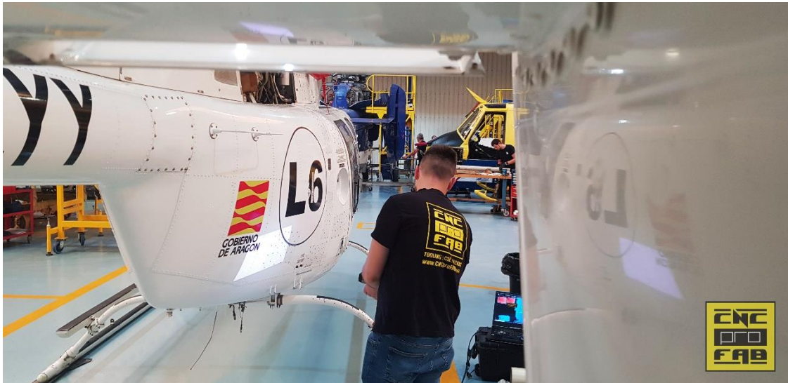
Bell 407 3D Scanning Process
